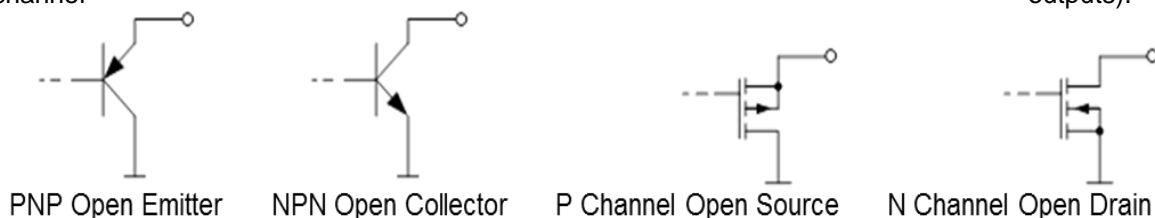
Figure 24 — Open-circuit Low Side Driver Type
